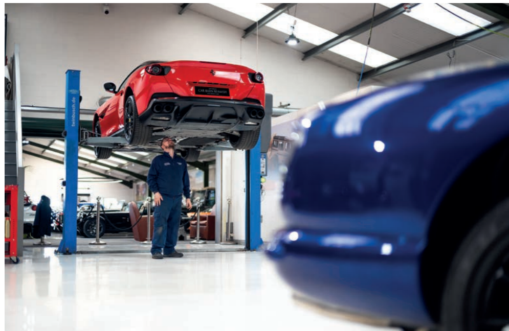
Above: The Car Barn Beamish workshop features four two-post ramps, with three technicians on hand for service, restoration and specialist repair work.
